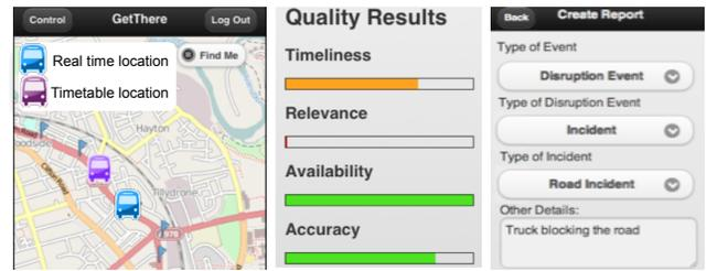
**Figure 2: Screenshots of the *GetThere* smartphone app showing (left to right): vehicle locations; the results of invoking the quality assessment service; and creating a disruption report.**
